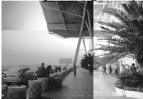
**Fig.** An intermediate image showing independently equalized sectors. Note intensity differences along the sector boundaries
