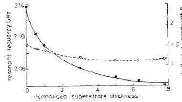
Figure Variations of resonant frequency and bandwidth with dielectric thickness
