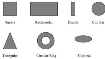
Figure: Various microstrip patch configurations
