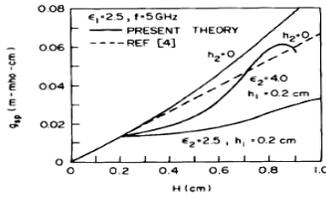
Figure Variations of space wave conductance's with substrate and dielectric thickness ( $a = 1.1$  cm,  $f = 5$  GHz)
